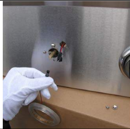
Disconnect the Wire and Change New LEDs
